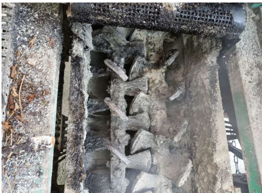
Figure 6.12 – Malaxeur (Source: Colas Belgium SA)
