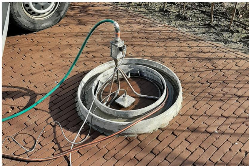
Figure 10 - Essai double anneau
