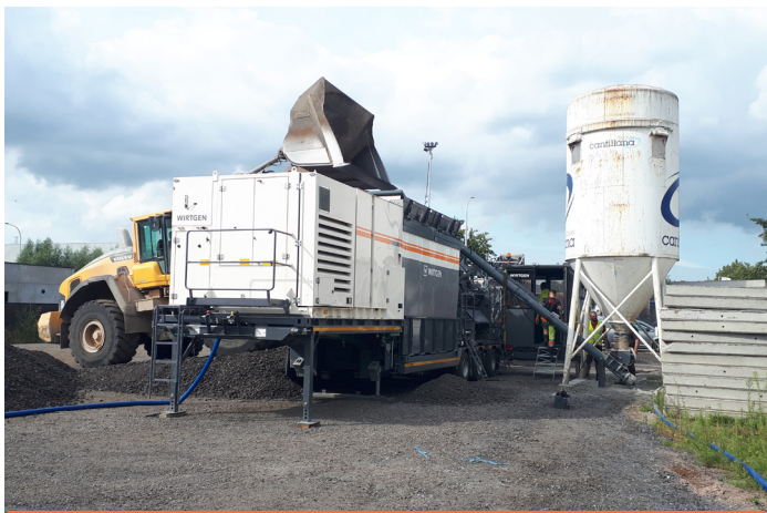
Figure 5 – Centrale de production mobile KMA240
