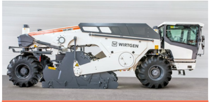
Figure 3 – Recycleur in situ (Source: Wirtgen)
