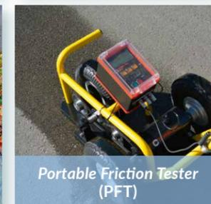
Portable Friction Tester (PFT)
