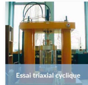
Essai triaxial cyclique
