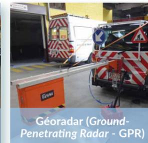
Géoradar (Ground-Penetrating Radar - GPR)
