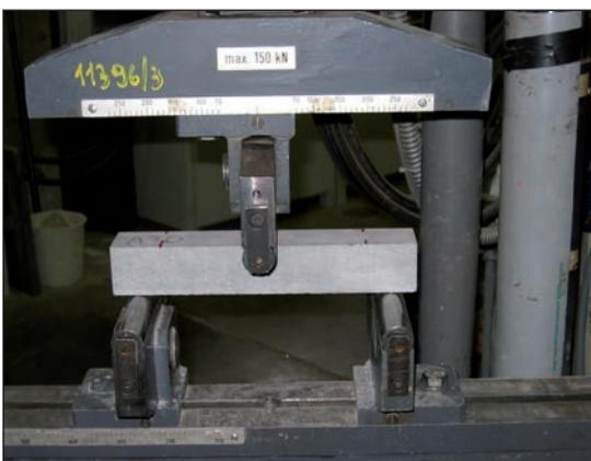
Figure 2.5 – Essai de flexion (Photo: CSTC)
